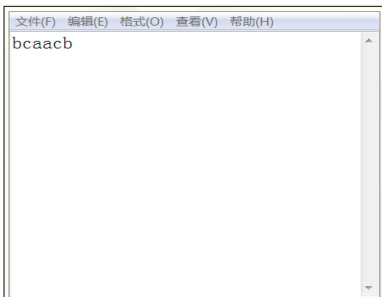
As shown in the [Figure 3-7. HID keyboard output](#), after open the text editor, press the corresponding key on the development board, the text editor will print the corresponding character.
