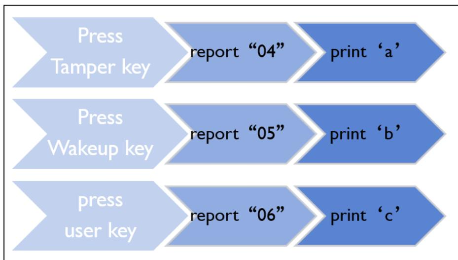
After the enumeration of HID keyboard devices completed, a keyboard device is added to the device manager of the host. As shown in the [Figure 3-6. HID keyboard applicaton example](#), Press the Tamper key of the development board, set the value of hid->data [2] to "04", send the message to the host through the device IN endpoint, and the host displays "a"; press the Wakeup key, and the host displays "b"; press the User key, and the host displays "c".
