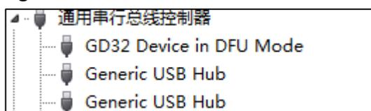
During the period of excuting download function, the host sends data to the DFU device through the USB bus, and then loads the data to the storage media. During the period of excuting upload function, the host receives the data from the DFU device through the USB bus and generates the bin file.
