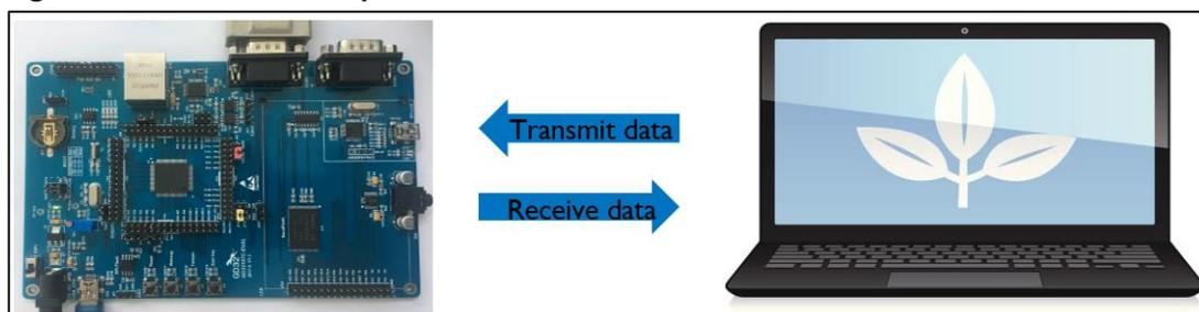
As shown in [Figure 3-19. Virtual serial port data interaction](#), CDC device implemented data callback function. When host sent the data to device, computer software transmit data to OUT endpoint of CDC device through USB bus, OUT endpoint load the received data into application buffer. When device sent the data to host, the data in application buffer is loaded into Tx FIFO, CDC device send the received data to host through IN endpoint, the received data is displayed in HyperTerminal.
